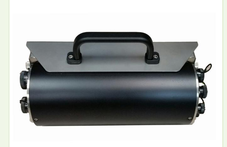
The Affinity delivers low-power, high-quality digitisation with full 24-bit resolution. Designed for data quality and durability, the Affinity is a stable and robust Linux-powered unit with onboard storage and networking facilities. An advanced module directly controls power supply to peripherals and reports their voltages via state-of-health communications.
