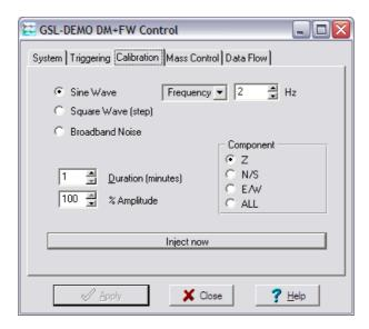
2. Select the calibration channel corresponding to the instrument, and choose **Broadband Noise.** Select the component you wish to calibrate, together with a suitable duration and amplitude, and click **Inject now**. A new data stream, ending  $C\underline{n}$  ( $\underline{n} = 0 - 7$ ) or MB, should appear in Scream!'s main window containing the returned calibration signal.
