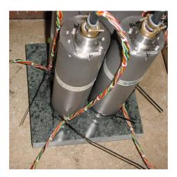
Placing a granite plinth on a sand layer increases the contact between the ground and the plinth, and improves the performance of the instrument. There is also no need to mix concrete or to wait for it to set, as in step 4.
