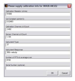
Most data can be found on the calibration sheet for your sensor. Under *Instrument response*, you should fill in the sensor response code for your sensor, according to the table below. *Instrument Type* should be set to the model number of the sensor.
