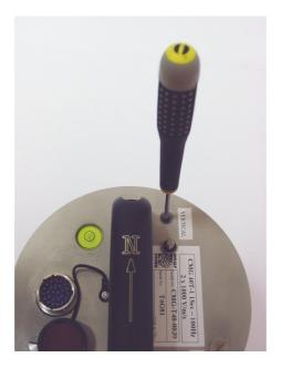
5. Turn the pot either way until the offset readout is as close to 0 V as possible.
