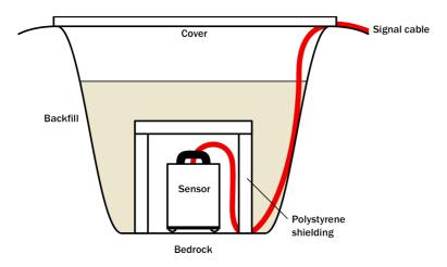
Depending on the time and resources available, this type of installation can suit all kinds of deployment, from rapid temporary installations to medium-term telemetered stations.
