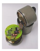
The steel sensor housing can be removed with an Allen key.
