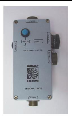
The breakout box also provides a standard Güralp power connector on a 10-pin mil-spec plug. The 40T draws a nominal current of 48 mA from a 12 V supply when in use; thus, using a 12 V, 25 Ah sealed heavy-duty lead-acid battery, you should expect the instrument to operate for around a week without recharging.
