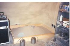
Again, this method produces inferior bonding to the instrument, and moisture becomes trapped between the hard surfaces. We recommend the use of fine dry sand (right) contained in a box if necessary, which can also insulate the instrument against convection currents and temperature changes. Sand has the further advantage of being very easy to install, requiring no preparation.
