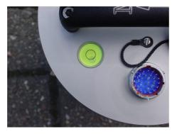
2. Unscrew the vent cap on the lid to allow the air pressure to equalise.
