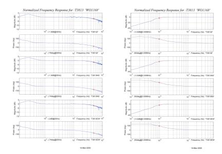
If you want to repeat the calibration to obtain more precise values at a frequency of interest, or to check that a sensor is still functioning correctly, you can inject calibration signals into the system using a Güralp digitizer or your own signal generator, and record the instrument's response.
