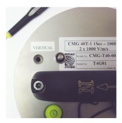
4. Insert the screwdriver through the opening, and engage the pot. An LED flashlight may be useful for locating the head.
