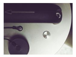
3. Using an Allen key, remove the screws holding the digitizer module onto the sensor.
