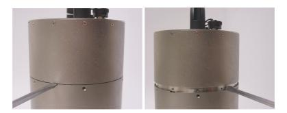
5. Carefully lift off the digitizer module, and unplug the ribbon cable from the sensor electronics.
