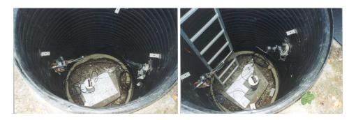
However, noise tests show that this method of installation is significantly inferior to the same concrete plinth with the tiles removed (right). Horizontal sensors show shifting due to moisture trapped between the concrete and tiling, whilst the vertical sensors show pings as the tile settles.
