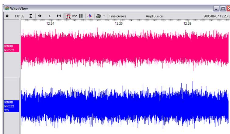
3. Open a Waveview window on the calibration signal and the returned streams by selecting them and double-clicking. The streams should display the calibration signal combined with the sensors' own measurements. If you cannot see the calibration signal, zoom into the Waveview using the scaling icons at the top left of the window or the cursor keys.
