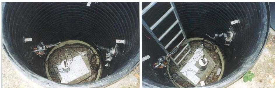
However, noise tests show that this method of installation is significantly inferior to the same concrete plinth with the tiles removed (right). Horizontal sensors show shifting due to moisture trapped between the concrete and tiling, whilst the vertical sensors show pings as the tile settles.
