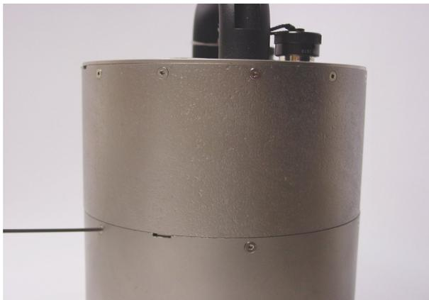
4. Place a flat-head screwdriver in the notches provided, and twist to lever off the digitizer module.
