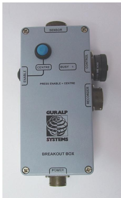
The breakout box also provides a standard Guralp power connector on a 10-pin mil-spec plug. The 40T draws a nominal current of 48 mA from a 12 V supply when in use; thus, using a 12 V, 25 Ah sealed heavy-duty lead-acid battery, you should expect the instrument to operate for around a week without recharging.
