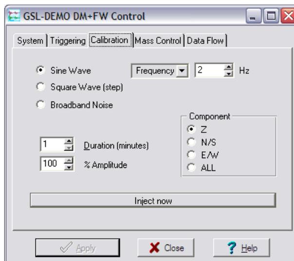
2. Select the calibration channel corresponding to the instrument, and choose **Broadband Noise**. Select the component you wish to calibrate, together with a suitable duration and amplitude, and click **Inject now**. A new data stream, ending  $C_n$  ( $n = 0 - 7$ ) or MB, should appear in Scream!'s main window containing the returned calibration signal.
