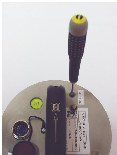
5. Turn the pot either way until the offset readout is as close to 0 V as possible.
