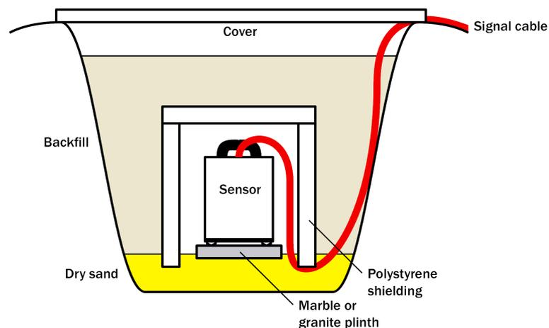
4. Pour a layer of loose, fine sand into the pit to cover the base. The type of sand used for children's sand-pits is ideal, since the grains are clean, dry and within a small size range. On top of the sand, place a smooth, flat granite plinth around 20 cm across, and shift it to compact the sand and provide a near-level surface.
